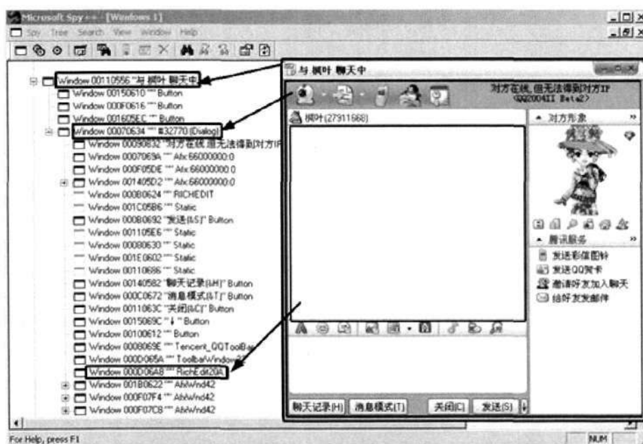
Figure 4-14: QQ chat interface and window class inspected by Spy++.
