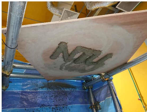
76 Fig. 1 NTU logo manufactured by overhead spray-based 3D printing
