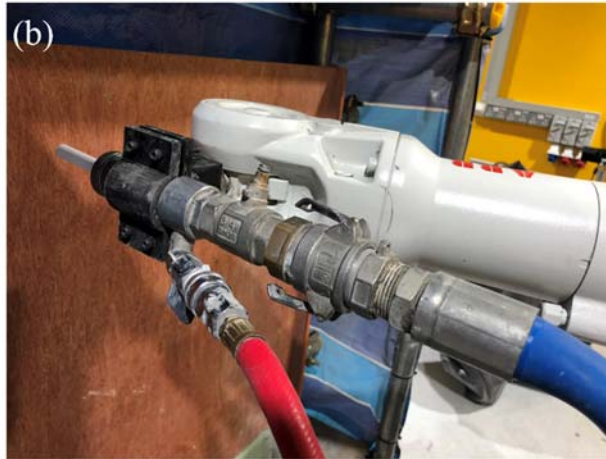
Fig. 6 Setup of spray tests: (a) equipment setup; (b) details of spray nozzle
