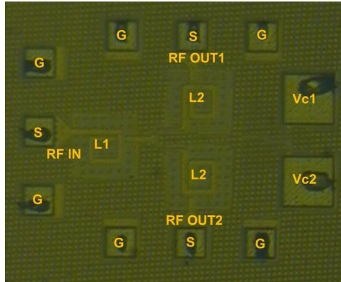
Figure 5-12 Photography of the designed SPDT switch
