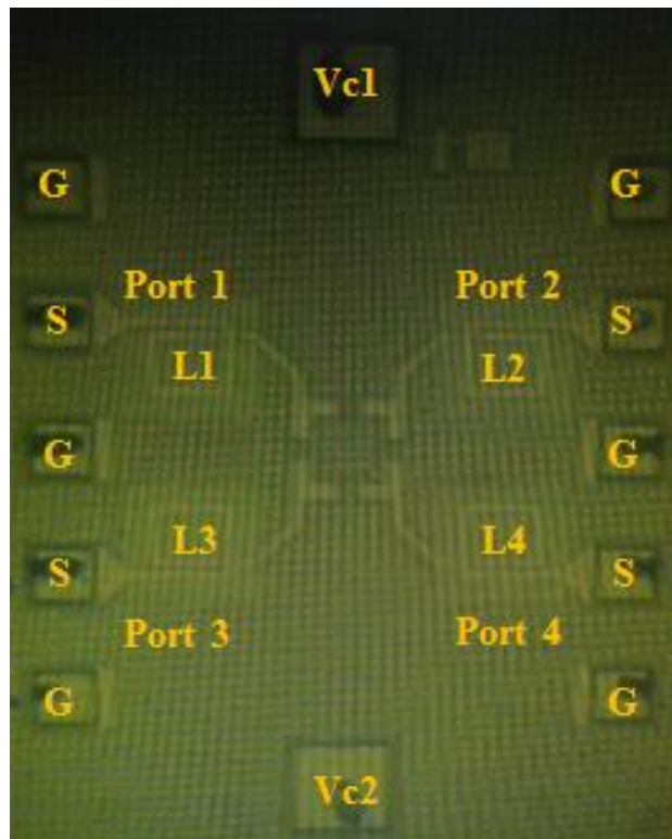
Figure 7-7 Photography of the designed DPDT Switch
