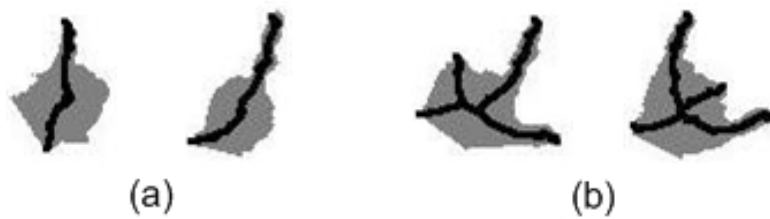
Figure 3.16: Some confusing cases for skeleton matching [3], where very different shapes can lead to similar skeletons.
