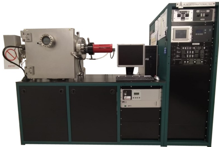
Figure 28: AJA ion beam etching system with a secondary ion mass spectrometer (SIMS) end point detector.
