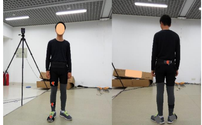
Fig. 6. Experiment Setups: IMU and Optical System
