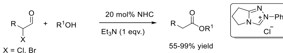
Scheme 1.24 Rovis' NHC-catalyzed self-redox reaction
