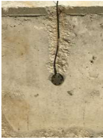
c) Mounted pressure transducer
