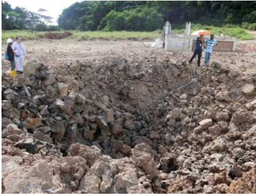
Figure 5.40 Crater formation resulted from 50kg TNT buried and detonated below 1.4m deep
