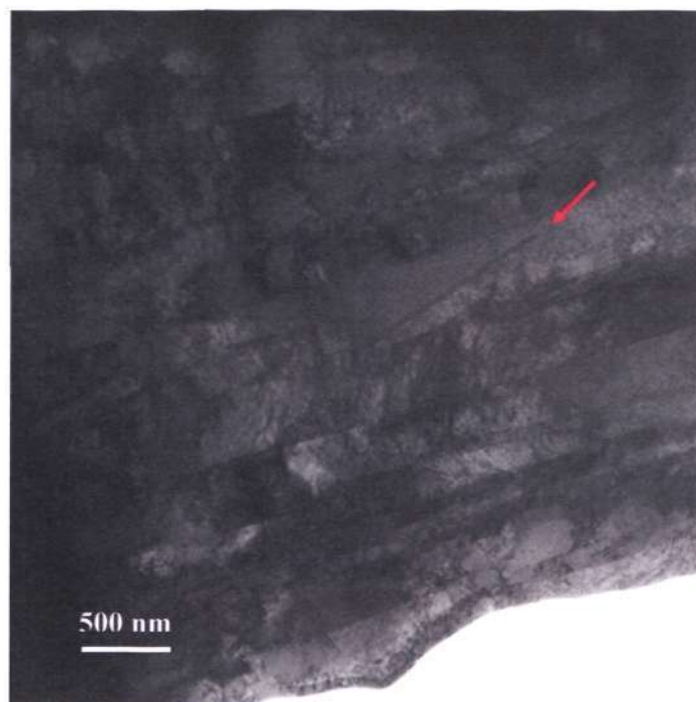
Figure 5-20 TEM image of Au 250 Ca at lower magnification, showing the appearance of one twin.
