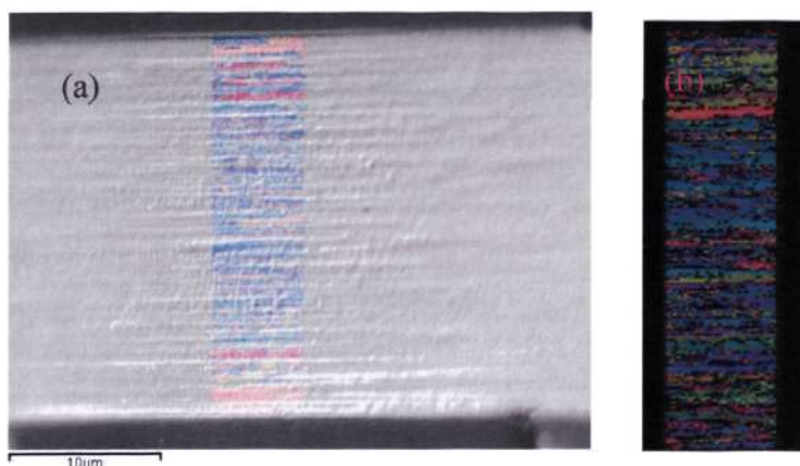
Figure 3-6 (a) Superimpose of orientation imaging map (OIM) onto the SEM captured microstructure and (b) OIM alone.
