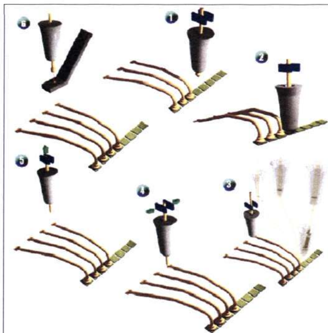
Figure 2-3 Basic gold ball wire bonding cycle (Small Precision Tool, 2009).
