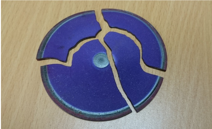
Figure 3.14 - Picture of LaB6 target that cracked due to the different coefficient of thermal expansion between the target, the copper magnetron and the Mo target holder.
