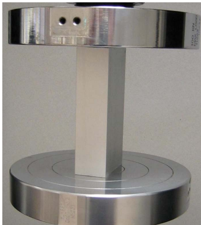
Figure 8.8 A bonded Al tube filled with Alporas foam during compression testing.
