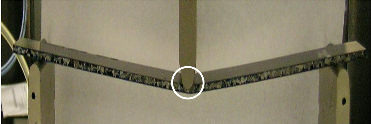
Figure 5. 5 In-Situ picture of the sandwich beam specimen failed by face sheet cracking (geometry – 1) at a displacement of 14.8mm.
