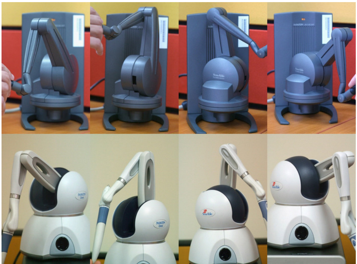
Figure 7.13 Synchronized motion of the haptic devices associated with the same tool object
