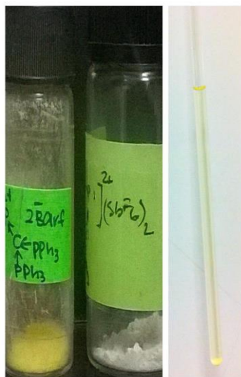
Figure 20. Color change as a result of interion contacts in [3c][\text{SbF}_6]_2 and [3c][\text{BAr}^f_4]
