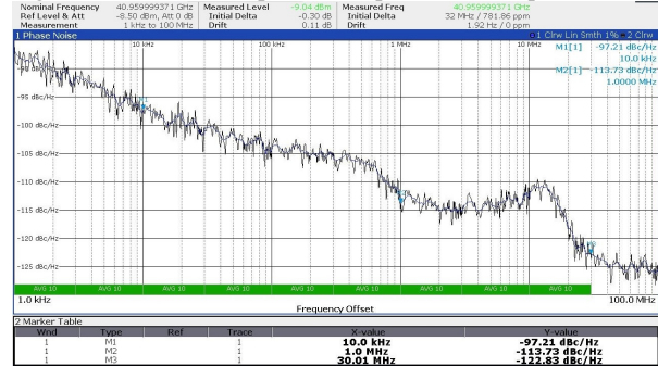
Fig. 6. Measured phase noise at 40.96 GHz.
