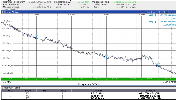
Fig. 9. Measured PLL phase noise at 311.55 GHz.
