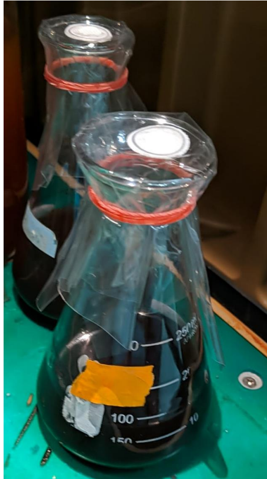
Figure 3. 6 Decolorization assay performed in conical flasks incubated in a temperature-controlled incubator
