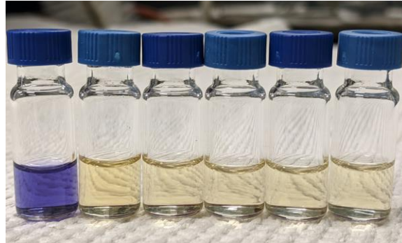
Figure 4. 5 Decolorized AB113 samples (0 h, 12 h, 24 h, 36 h, 48 h, 60 h (from left to right))
