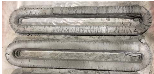
590 Fig. 13 Defects due to poor pumpability
