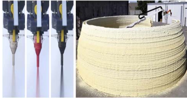
540 541 Fig. 12 3D printing of foam concrete materials [75] . Reproduced from Ref. [75] with permission © 542 American Association for the Advancement of Science.
