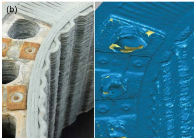
Fig. 2 Concrete Printing [16, 17] : (a) gantry framework; (b) details of printed structure and scanned surface; (c) layered texture in printed structure by similar gantry-based printing system. Fig. 2 (a) and Fig. 2 (b) are reproduced from Ref. [16] with permission from IAARC.
