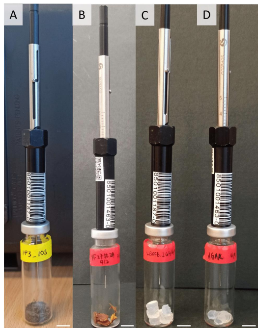
Figure 8: SPME fibre assembly set-up for collection of sample analytes. A: F. siamensis sample with one cut plug with 1 g of autoclaved sieved soil; B: F. siamensis sample with six cut plugs; C: R. microporus sample with six cut plugs; D: PDA sample with six cut plugs. Scale bars are 10 mm.
