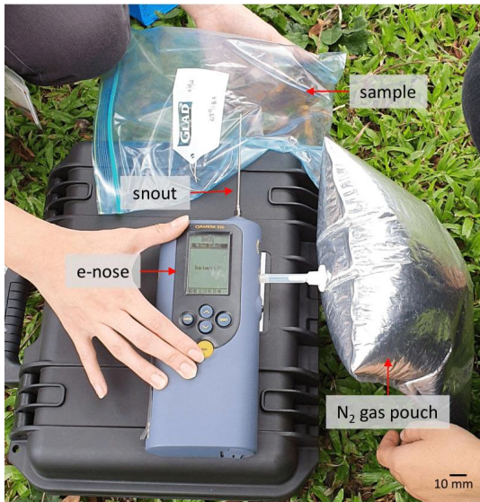
Figure 22: E-nose set-up of the real time field prediction of unknown sample with nitrogen gas used as the baseline gas. Adapted from Tan et. al [81].
