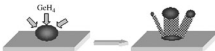
Figure 3.1 Growth of GeNW on catalyst (black color) via VLS method. [Reproduced with permission from ref. (116). Copyright 2005 Wiley-VCH Verlag GmbH & Co. KGaA, Weinheim]
