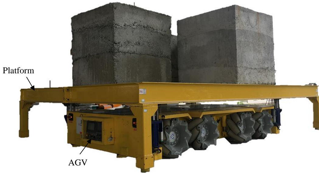
Figure 9. Platform and AGV
