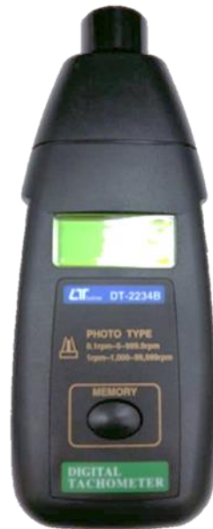
Figure 7.4 Contactless tachometer for measuring compressor shaft speed
