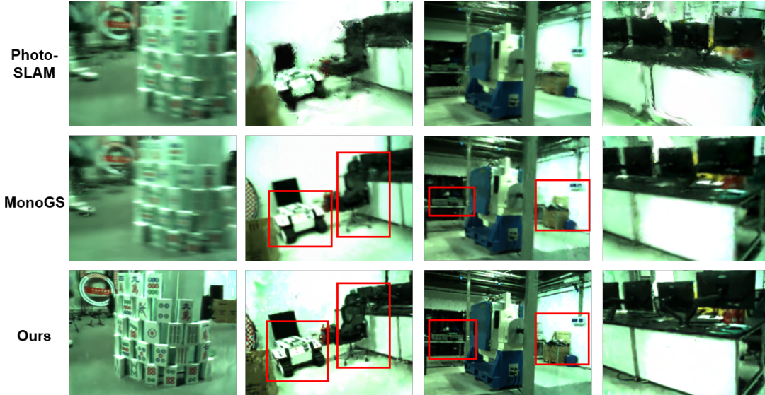
Fig. 4: Comparison of rendering quality on the DEVD dataset. Our method can achieve sharper reconstructions.
