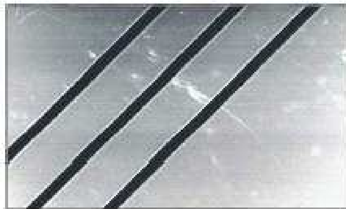
Figure 2.6 A Chrome-on-Quartz Photomask where the Chrome has been Removed using a Femtosecond Laser [13]
