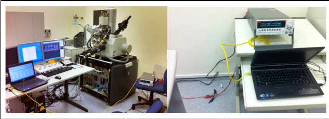
Figure 3.7 In-situ electromigration dual beam FIB setup.
