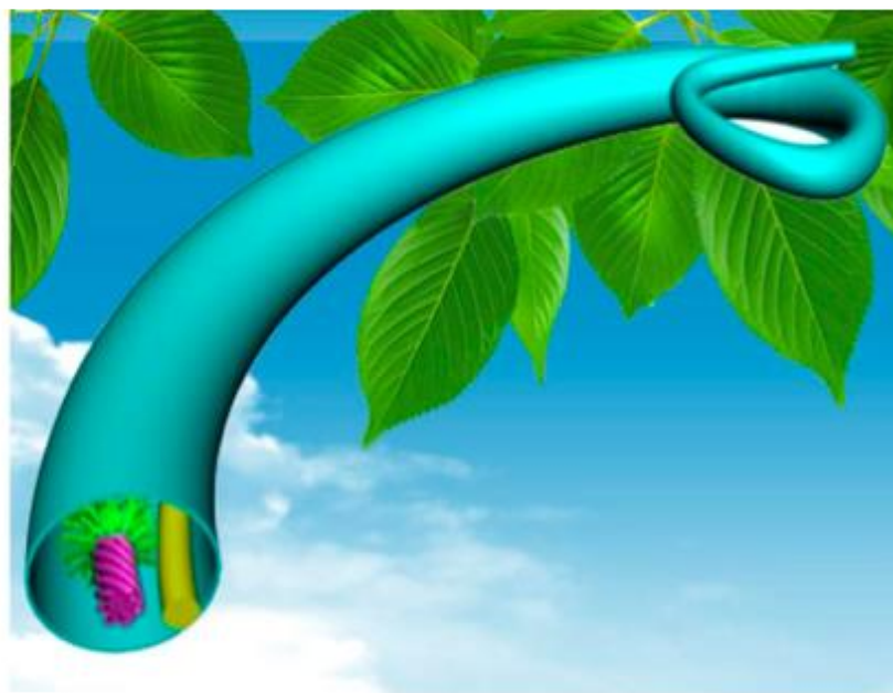
Figure 3-17 Schematic illustration of the fiber-shaped Ni-Zn battery.
