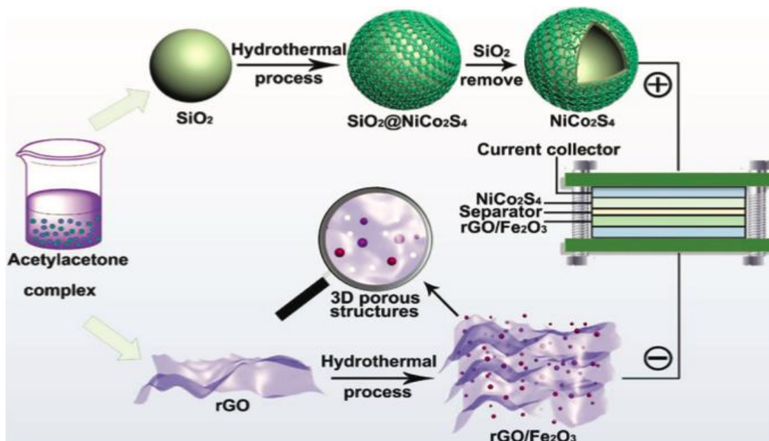
Figure 2-16 Schematic illustration on how to form NiCo 2 S 4 hollow spheres and 3D porous rGO/Fe 2 O 3 hybrid structures as well as the device fabrication.[84]
