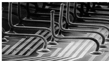
Figure 2.11 S-shaped micro-spring interconnects by Form Factor (Garrou, 2000)
