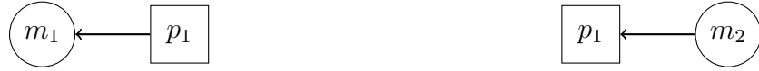
(a) Material m_1 is produced by plant p_1 , such that m_1 has output dependency on p_1 . (b) Material m_2 is processed at plant p_1 , such that p_1 has input dependency on m_2 .
