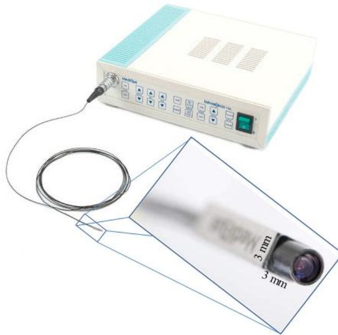
Fig. F.1 Photograph of micro ScoutCam™ 3.0 and processor.
