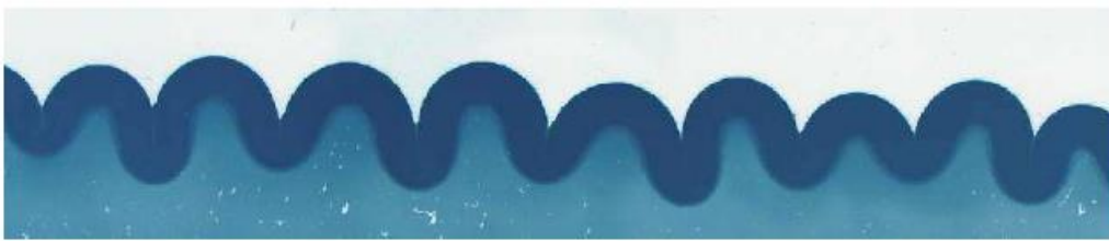
Figure 1-6: Buckling of a gel film attached to a compliant substrate. Reproduced from Sultan and Boudaoud (2008)
