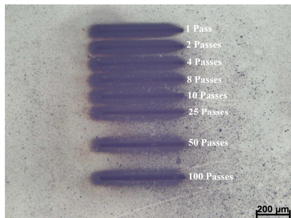
Figure 5.19: Low magnification of Fs laser ablated grooves machined using different number of cutting pass for a fluence of 12.5 \text{ J/cm}^2 .
