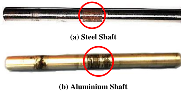
Figure 3.12: Wear of Metal Shafts with Chrome Steel Test Piece
