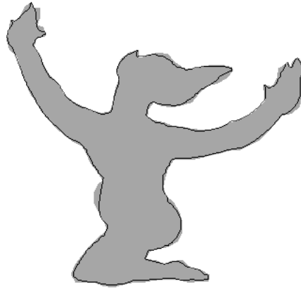
Figure 5.7: Superimposed original image and vectorized image (original image in shadow and vectorized image in outline)
