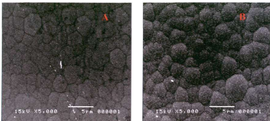
Figure 3-26 SEI fractographs taken at a higher magnification. (Left) Surface A at the central region. (Right) Surface B at the bare gold substrate
