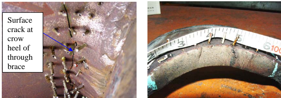
(a) Close-up view and opened surface crack at crown heel of through brace of Specimen SI
