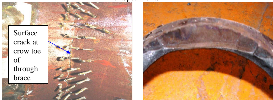
(a) Close-up view and opened surface crack at crown heel of through brace of Specimen SI
