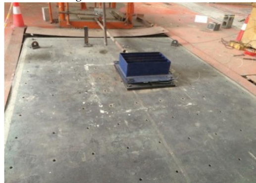
(b) Photograph of tuned liquid damper (TLD) specimen and shear force measurement table
