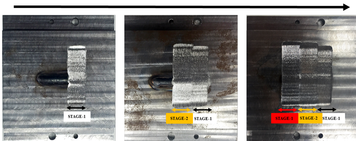
Figure 7.3: Stage-wise weld seam removal from workpiece surface in dry conditions.
