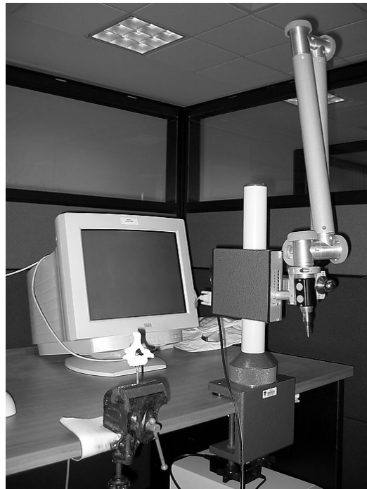
Figure 51: Digitizer FaroArm setup.
