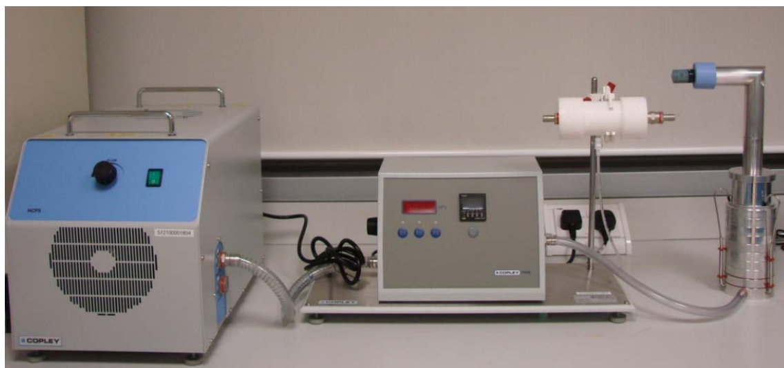
Figure 3.9 Experimental set up for the in vitro inhalation experiments using ACI.
