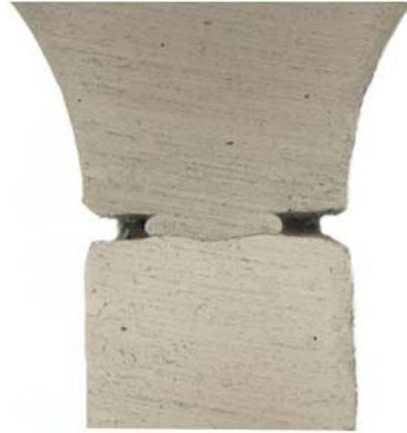
Fig. 5-17 SEM micrograph of the joint interface after energy director melting
