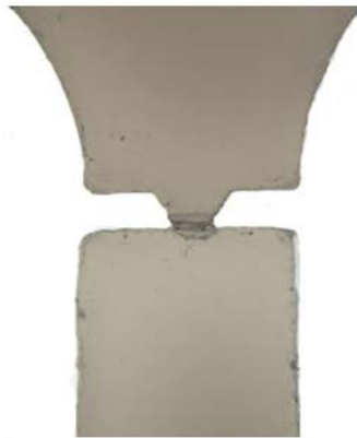
Fig. 5-16 SEM micrograph of the joint interface after plastic deformation
