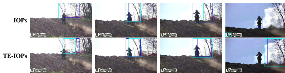
Fig. 5.7 Some failure cases of our TE-IOPs. Only top 2 proposals are shown for clarity. The four frames are from the same video playing from left to right. In the fourth frame, our method assigns higher spatiotemporal objectness scores to the noisy detections due to the strong and consistent noisy detections in previous frames.
