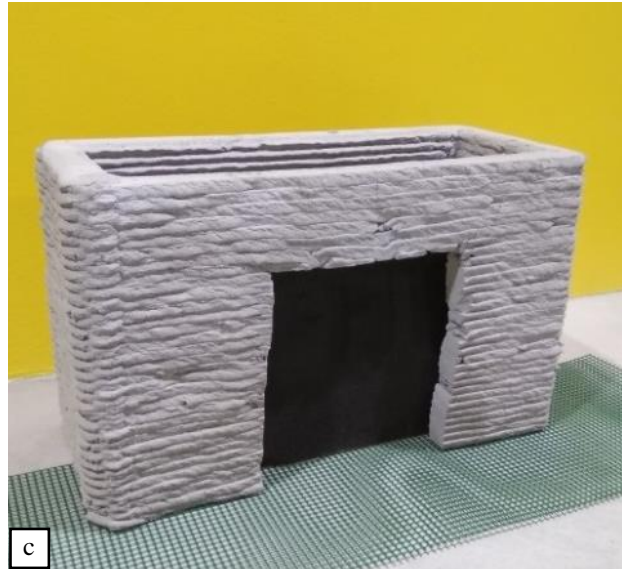
Figure 5.13: (a) Printing with supports (b) before post-processing (c) after post-processing
