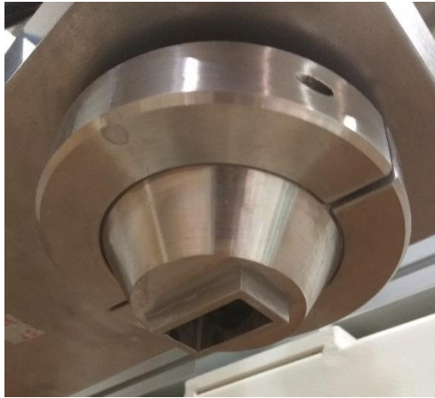
Figure 5.2: 30 mm by 15 mm nozzle used for printing
