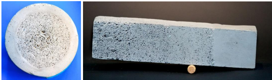
Figure 2.24: Radial and linear density gradient of concrete samples [86]
