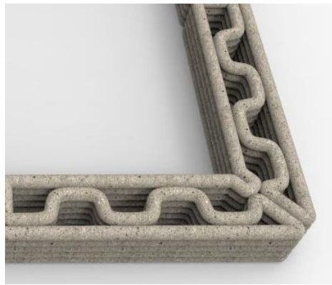
Figure 7.2: Lattice designed for PBU printing.
