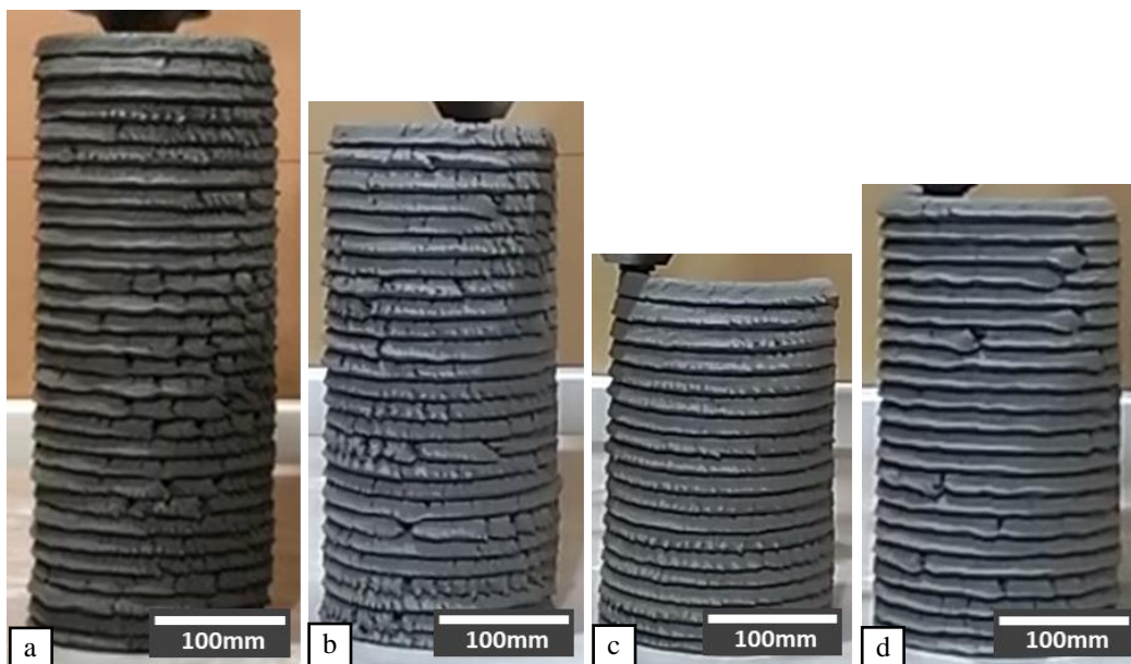
Figure 3.16: Maximum layers printed for the different mixture (a) Mix 3; (b) Mix 12; (c) Mix 8; and (d) Mix 23
