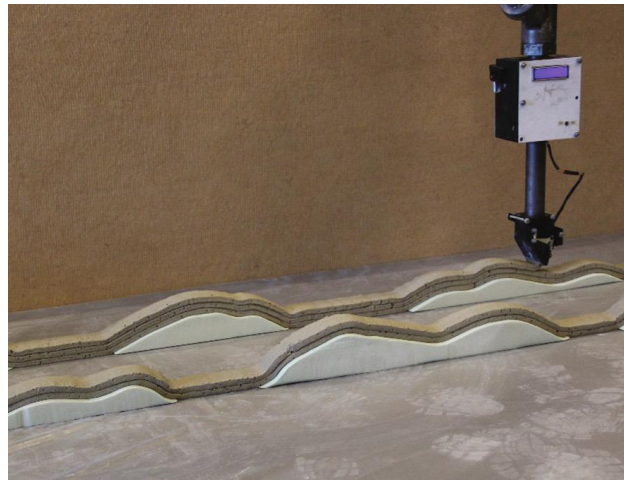
Figure 2.8 Printing along the arbitrary curved profile without predetermining nozzle variation in height position [27]
