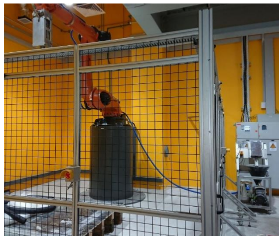
Figure 7.1: Robotic arm printer used for large scale printing
