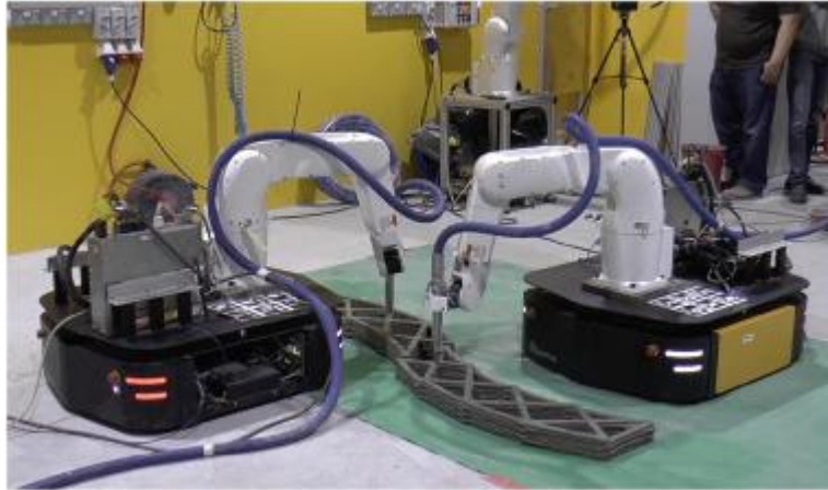
Figure 2.10 Concurrent printing of a single structure by 2 mobile robots [37]
