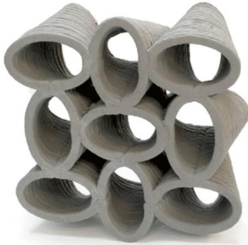
Figure 2.14. Concrete printed acoustic wall element [41].
