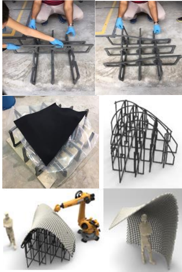
Figure 2.13. Curved bed printing with printed frames printed in SC3DP, NTU.
