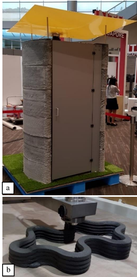
Figure 2.15. (a) 3D printing of modular toilet with high volume fly ash at SC3DP, NTU. (b) 3D printing of geopolymer [44].
