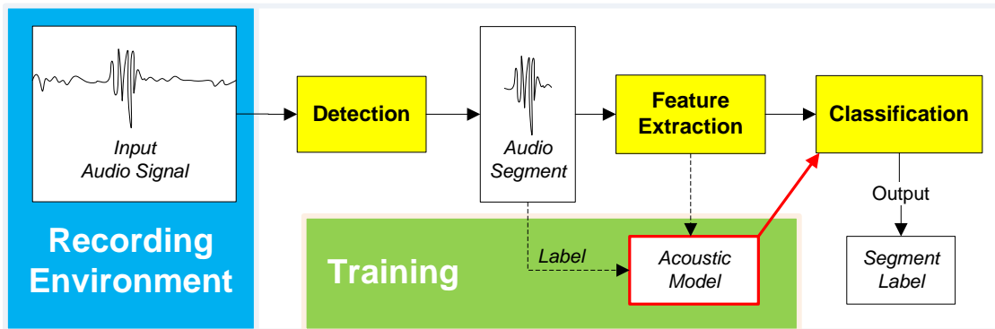
Figure 2.4: The structure of a typical sound event recognition (SER) system
