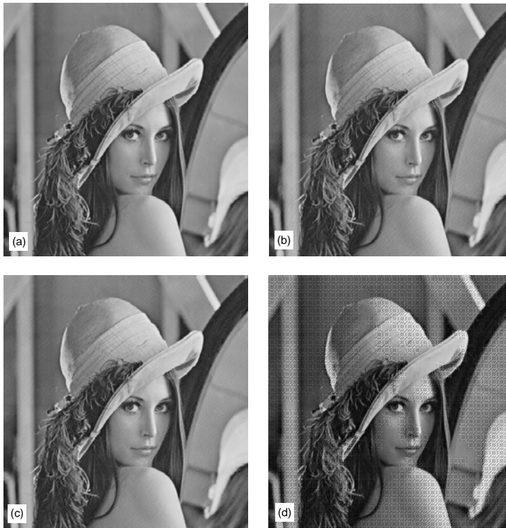
Fig. 5: (a) The original image of Lena, the watermarked images of Lena using (b) SCHT with PSNR = 39.95 dB, (c) DFT with PSNR = 37.72 dB, and (d) UCHT with PSNR = 26.41 dB.
