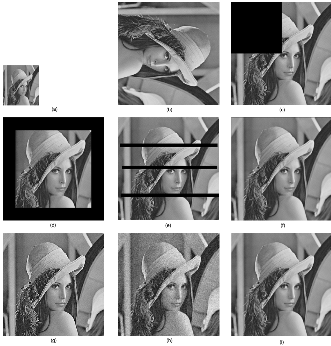
Fig. 6: The SCHT watermarked images subjected to various attacks: (a) The resized, (b) the rotated, (c) the cropped (a quarter image), (d) the cropped (central portion remained), (e) the painted, (f) the filtered, (g) the sharpened, (h) the noised, and (i) the phase perturbation attacked.
