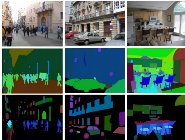
Figure 2.12: Examples of annotation on images of ADE20K. Multi-layer structure is used for storing the maps of same image[8].
