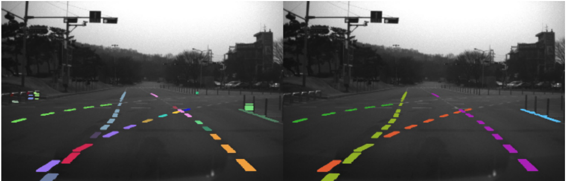
Figure 2.22: Result of CRF clustering. Left is coarse clustering and right is refined clustering.[11]
