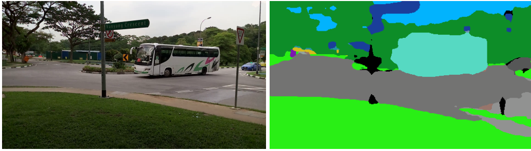
Figure 2.8: A initial result of scene recognition with FCN based on pascal-context dataset. The process is done without any post-processing.
