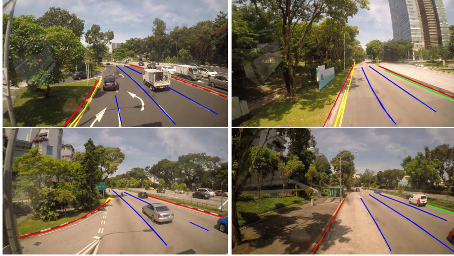
Figure 4.3: Examples of the representing curves on the dataset. Red: Road edge; Yellow: Double solid lane; Blue: Dashed lane; Green: Solid lane.
