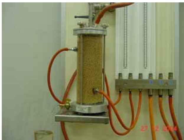
Figure 7.5 Experiment setup of a permeability test
