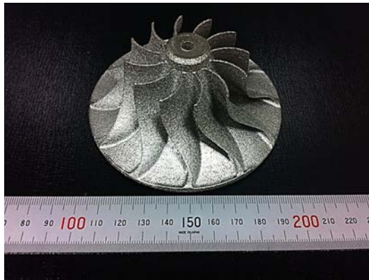
Figure 4. Photograph of the built impeller by using EBM
