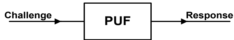
Figure 4: Challenge-Response pair definition for PUF
