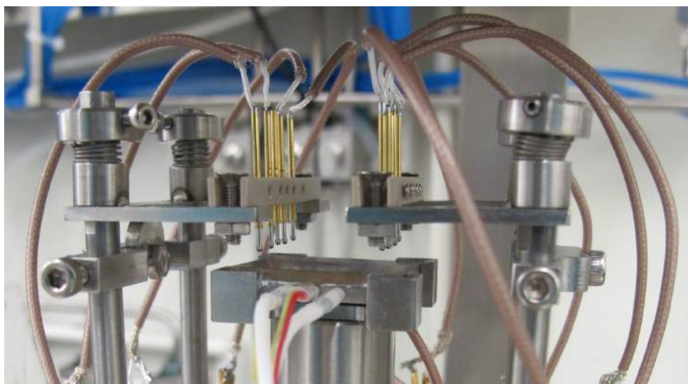
Figure 2.15: Image of the mounting element that the gas sensor is inserted into for characterization measurements.
