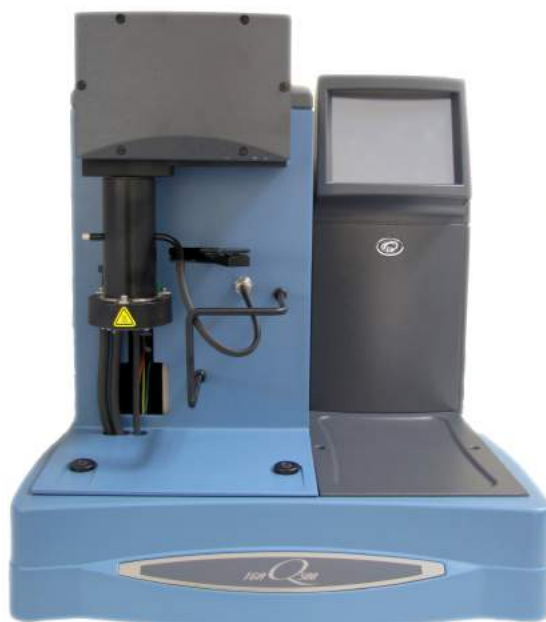
Figure 2.17: TA Instruments Q500 Thermogravimetric Analyser
