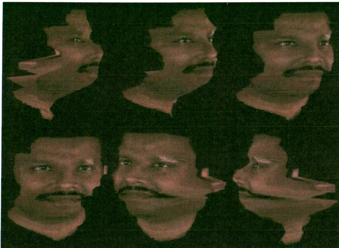
Figure 6.13: Result of 3D correlation window with fixed normal, fixed size and without visibility check
