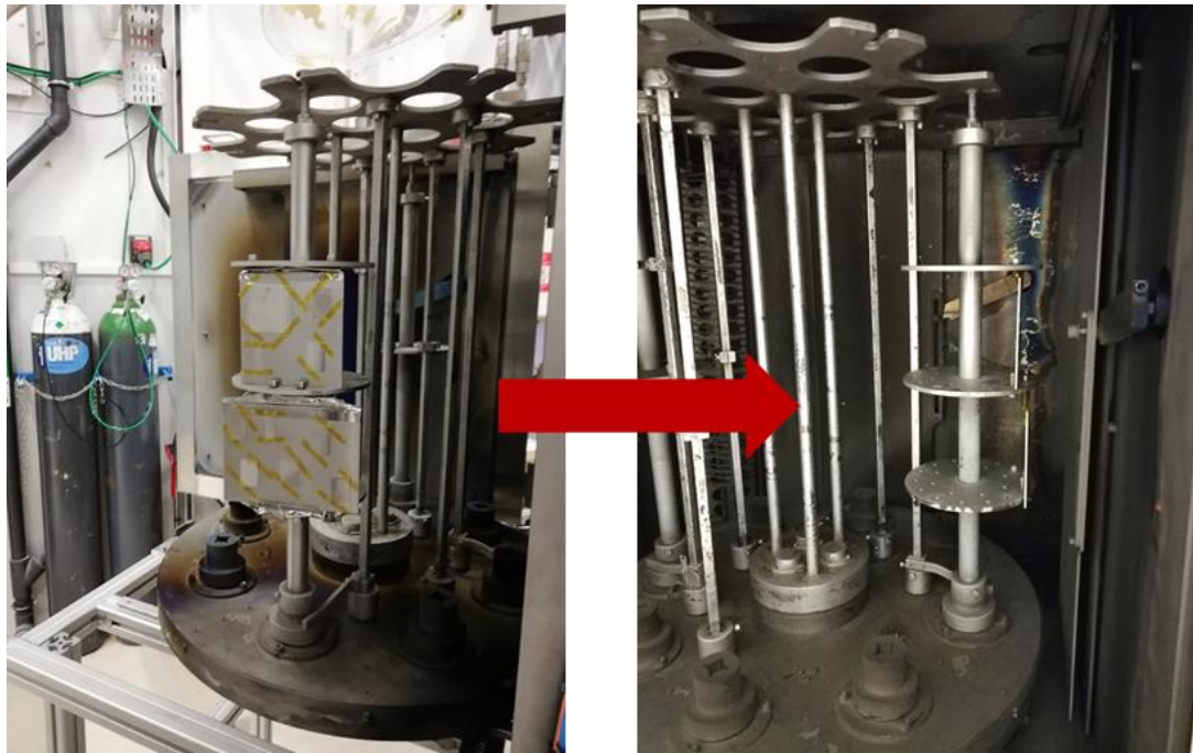
Figure 5: Substrates arrangement in the chamber for the aluminum plate technique
