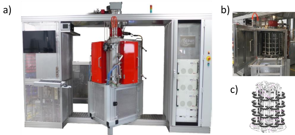
Figure 2: Photographs of the a) inside, b) outside of TriPros reactor and c) drawing of the substrate-holder.
