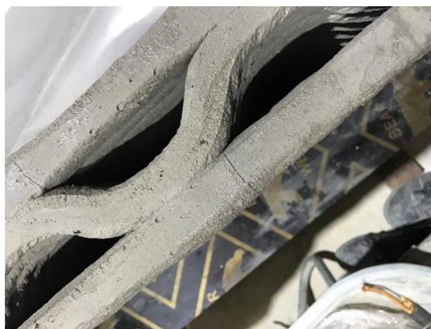
Figure 1 Cracks form on the surface of the printed structure
