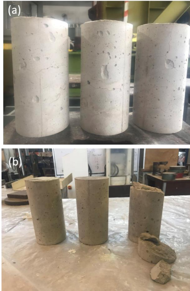
234 Figure 10 Results of spalling test: (a) 3DPFRCC; (b) 3DP plain concrete
